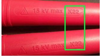
All 6550 and 6555 Models with firmware version 2.1/2.1 or later allow you to select  $0k\Omega$  or  $44k\Omega$  lead compensation before using the meter. Users with K22 marked leads should enable  $44k\Omega$  lead compensation on their 6550/6555. By default, all new products are shipped with K22 leads and  $44k\Omega$  lead compensation selected.
