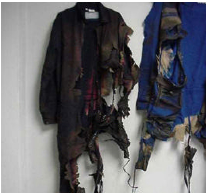
Figure 2: Two Layers of FR Coveralls after the Floor Level Arc Flash Incident
