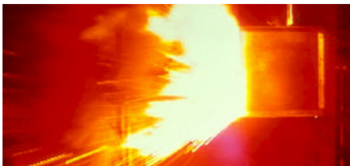
Figure 3: Arc-In-A-Box Flash Incident
