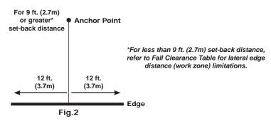
Install the leading edge self-retracting lifeline to the approved anchorage/anchorage connector by the anchorage attachment using a locking carabiner or other Honeywell approved connector. Verify that the snap hook is completely closed and locked.
