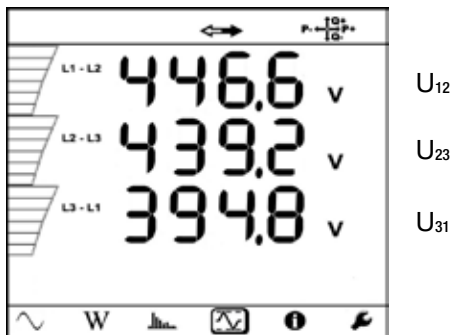
Maximum line voltage (3-phase 3-wire)
